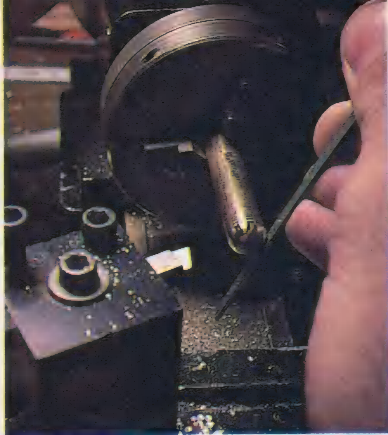
The end of the ball is rounded with a file.
